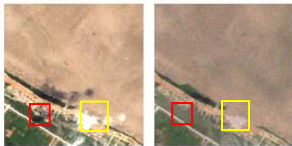
Figure 4. Result of Jiujiang's patch image in detail (red box: shadowing, yellow box: cloud)
